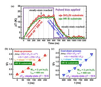
Fig. 7. (a) Transient  $\Delta T$  results and comparison with different substrates. Roughly 325 ns is needed to reach steady-state in both cases. Time constant extraction of (b) heat-up and (c) cool-down processes from the transient  $\Delta T$  measurement results with HR Si substrate of Fig. 7(a). The  $t/\tau$  values are obtained by plugging the measured individual  $\Delta T(t)$  values into the indicated formulas.
