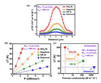
Fig. 4. (a) Cross sections of PD-normalized  $\Delta T$  of TG ALD  $\ln_2 O_3$  FETs with different substrates. (b)  $\Delta T$  extraction of TG ALD  $\ln_2 O_3$  devices with different substrates and power densities. Linear relationship is agreed in all the cases. (c) Comparison of the extrapolated  $\Delta T$  with different substrates given a constant PD.
