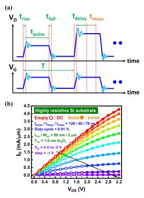
Fig. 8. (a) Diagram sketch of pulse measurement setup in time domain. The light blue damping illustrates the bias stabilization process after being set to desired values. (b) Output characteristics of a TG ALD  $\ln_2 O_3$  FET with short  $L_{\rm ch}$  of 80 nm and  $T_{\rm ch}$  of 1.9 nm on HR Si substrate achieving extremely high  $I_D$  up to 4.3 mA/ $\mu m$  with short-pulse measurement.
