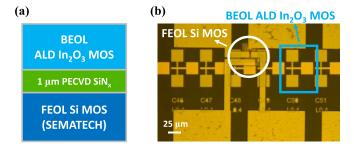
Fig. 9. (a) Structure illustration of combining BEOL ALD  $In_2O_3$  transistors and FEOL Si devices with 1- $\mu$ m-thick PECVD  $SiN_x$ . (b) Optical photograph of the structure in (a) where the indicated FEOL and BEOL devices are vertically separated by a 1- $\mu$ m-thick PECVD  $SiN_x$  layer.
