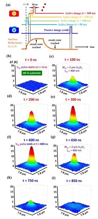
Fig. 6. (a) Working mechanism of transient thermal property study with an ultrafast HR TR imaging system. (b)–(i) Transient TR characteristics of a TG ALD  $\rm In_2O_3$  FET on HR Si substrate. The device was self-heated-up by applying a  $V_{\rm DS}$  pulse starting at 0 ns and ending at 600 ns. (b)–(e) Demonstrate the heat-up process while (f)–(i) demonstrate the cool-down process.
