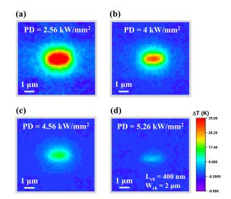
Fig. 3. SHE visualization of TG  $In_2O_3$  FETs in experiments with substrates of (a)  $SiO_2/Si$ , (b) sapphire, (c) highly resistive Si, and (d) diamond with various PD. The  $L_{\rm ch}$  and  $W_{\rm ch}$  are 400 nm and 2  $\mu$ m, respectively, for all the devices. The device on a  $SiO_2/Si$  substrate is the most self-heated while the one on a diamond substrate is the least.
