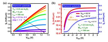
Fig. 5. (a) Output and (b) transfer characteristics of an  $In_2O_3$  FET with  $L_{ch}$  of 100 nm and  $T_{ch}$  of 2.5 nm on a diamond substrate, performing ultrahigh  $I_D$  of 3.7 mA/ $\mu$ m under dc condition.
