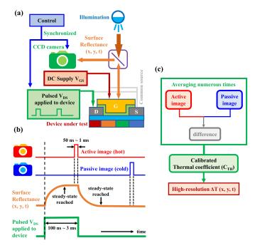
Fig. 2. (a) Schematic illustration of the ultrafast HR TR imaging system setup. (b) Working mechanism of the ultrafast HR TR imaging equipment in time domain. (c) Transformation from TR signal to a temperature scale.
